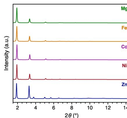
**Figure 1.** Powder X-ray diffraction patterns of activated  $M_2(olz)$  frameworks ( $M = Mg, Fe, Co, Ni$ ) and ethanol-solvated  $Zn_2(olz)$ ;  $\lambda = 0.72768 \text{ \AA}$ . The diffraction patterns are offset for clarity.
