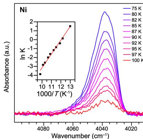
**Figure 4.** Enthalpy and entropy changes upon adsorption of  $\text{H}_2$  on the open metal site. Variable-temperature infrared spectra were collected for  $\text{Mg}_2(\text{olz})$  and  $\text{Ni}_2(\text{olz})$ , and the insets show the van't Hoff plots that were used to extract the enthalpy and entropy change in  $\text{H}_2$  upon adsorption to the open metal site.
