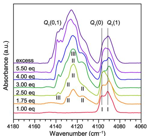
**Figure 3.** Hydrogen adsorbed at multiple sites as a function of loading. Infrared absorption of  $\text{H}_2$  in  $\text{Mg}_2(\text{olz})$  was performed at 15 K. The equivalents (eq) refer to the number of  $\text{H}_2$  molecules per Mg, and the spectral features corresponding to the distinct sites observed are denoted with Roman numerals.  $Q(0)$  refers to *para*- $\text{H}_2$  and  $Q(1)$  to *ortho*- $\text{H}_2$  modes.
