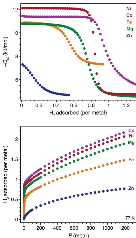
**Figure 2.** Top: isosteric heats of adsorption plotted as a function of the amount of  $H_2$  adsorbed for  $M_2(\text{olz})$ . Bottom: equilibrium  $H_2$  adsorption isotherms for  $M_2(\text{olz})$  at 77 K, where the amount adsorbed is plotted in terms of  $H_2$  molecules per metal atom.
