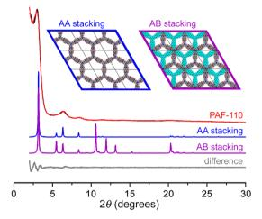
**Figure 3.** Experimental (black), refined (red), simulated AA stacking (blue), simulated AB stacking (purple), and difference (gray) powder X-ray diffraction patterns for PAF-110; (inset) illustration of the AA and AB stacking models for PAF-110. Cu Kα radiation was used.
