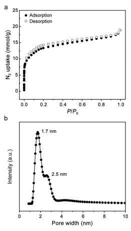
Figure 4. (a) Nitrogen isotherms and (b) the pore size distribution for PAF-110.
