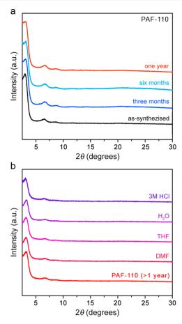
Figure 5. (a) Powder X-ray diffraction patterns for PAF-110 assynthesized and after air exposure for three months, six months, and one year. (b) Powder X-ray diffraction patterns for a sample of PAF-110 stored in air >1 year following treatment with various solvents and acid; samples were treated by soaking in a given solvent for 7 days at room temperature.
