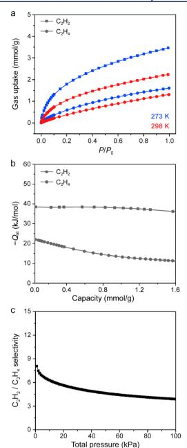
**Figure 6.** (a) Acetylene (squares) and ethylene (circles) adsorption isotherms for PAF-110 at 273 K (blue symbols) and 298 K (red symbols).  $P_0=1$  bar. (b) Isosteric heats of adsorption,  $Q_{\rm str}$  for acetylene and ethylene. (c) Acetylene/ethylene adsorption selectivity of PAF-110 at 298 K, as determined from ideal adsorbed solution theory.
