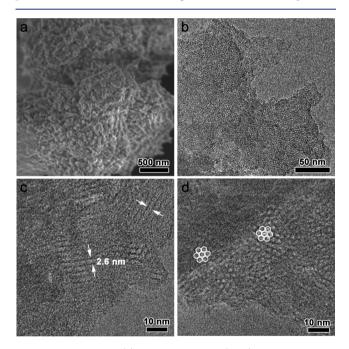
Figure 2. SEM image (a) and TEM images (b–d) of PAF-110. The white arrows in (c) highlight the straight channels with a diameter of  $\sim$ 2.6 nm, and the hexagonal pores are highlighted in (d).
